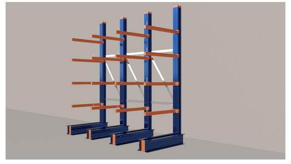
Type : **Cantilever Racking** Height: 5000mm Width: 3000mm Depth: 1200mm Paint: Blue and Orange. Corrosion resistant powder coat finish **Steel Construction** Base + 4no. Levels Capacity per shelf 850 kg UDL (Uniformly Distributed Weight) [Beam Thickness 100mm high 60mm wide] High stability / freestanding Adjustable Arms **Base Fixings Included**
