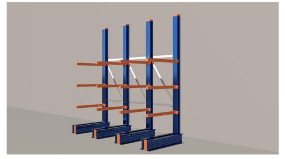
Type : **Cantilever Racking** Height: 5000mm Width: 4000mm Depth: 1200mm Paint: Blue and Orange. Corrosion resistant powder coat finish **Steel Construction** Base + 4no. Levels Capacity per shelf 850 kg UDL (Uniformly Distributed Weight) [Beam Thickness 100mm high 60mm wide] High stability / freestanding Adjustable Arms **Base Fixings Included**
