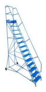
Type: Mobile Stairs Height: 4250mm Width: 1230mm (internally) - Each upright 50mm W Depth: 2470mm Paint: Steel. Corrosion resistant powder coat finish Steel Construction 13no. steps Working Height: 4250-5000mm Working Platform Height: 3250mm Colour: Blue
