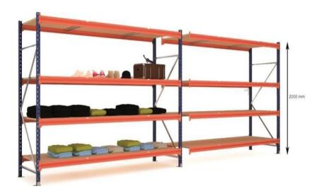
Type: Long span Shelving Height: 2000mm Width: 1800mm (internally) - Each upright 50mm W Depth: 800mm Paint: Orange/Blue. Corrosion resistant powder coat finish Steel Construction 3no. 22mm MDF Board Capacity per shelf 500 kg UDL (Uniformly Distributed Weight) Total load capacity of 2000 kg shelf UDL High stability / freestanding Starter & Extender bays
